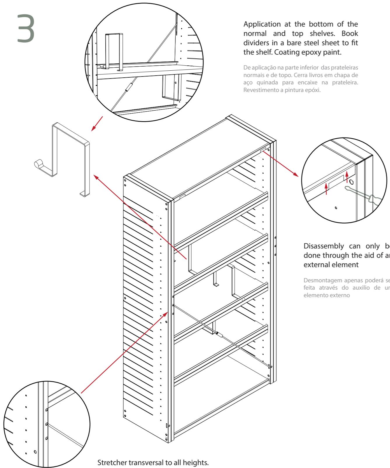
Application at the bottom of the normal and top shelves. Book dividers in a bare steel sheet to fit the shelf. Coating epoxy paint.
